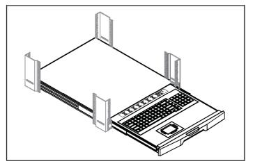
Figure 3. Fixing the keyboard drawer into the rack.
