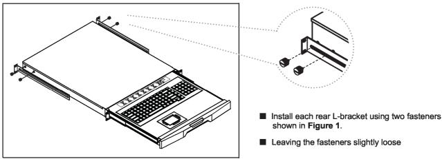
Figure 1. Installing the rear L-bracket to the keyboard drawer.
