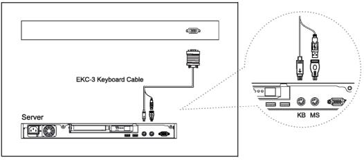
Figure 6. Example of connecting EKC-3 keyboard cable to server via PS/2 interface
