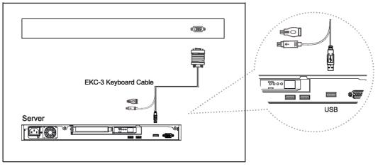
Figure 4. Example of connecting EKC-3 keyboard cable to server via USB interface
