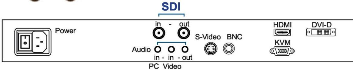
\*\*\* For SDI option, casing depth will be changed from 480mm ( 18.9" ) to 530mm ( 20.9" )
