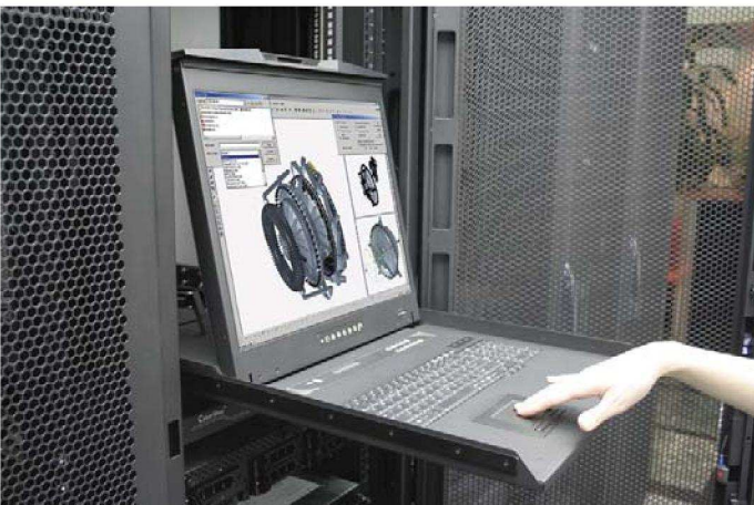
Figure 6. Operating the LCD keyboard drawer
