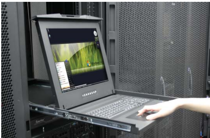
Figure 6. Operating the LCD keyboard drawer.
