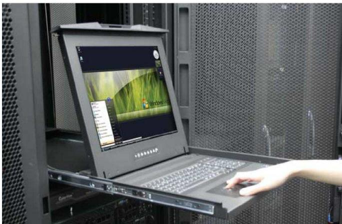
**Figure 6.** Operating the LCD keyboard drawer.
