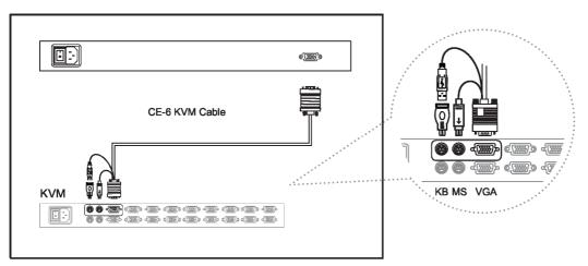
Figure 10. Example of connecting KVMCE-6 4-in-1 Combo KVM cable to KVM via PS/2 interface
