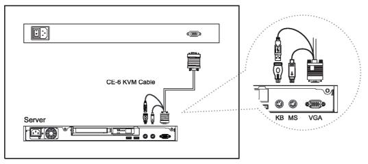
Figure 9. Example of connecting KVMCE-6 4-in-1 Combo KVM cable to server via PS/2 interface
