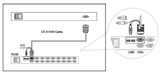
Figure 12. Example of connecting KVMCE-6 4-in-1 Combo KVM cable to KVM via USB interface
