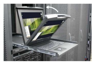
■ Flip up the LCD to a suitable angle shown in **Figure 5**.
