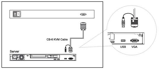
Figure 7. Example of connecting KVMCB-6 2-in-1 USB KVM cable to server via USB interface
