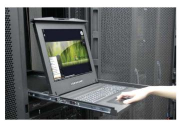
Figure 6. Operating the LCD keyboard drawer.
