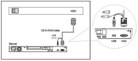
Figure 11. Example of connecting KVMCE-6 4-in-1 Combo KVM cable to server via USB interface
