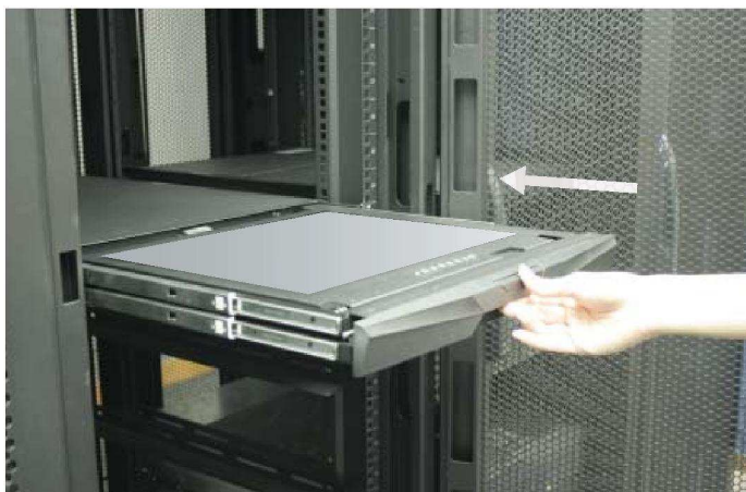
Figure 6. Sliding in the LCD keyboard drawer by pressing the carry handle button.
