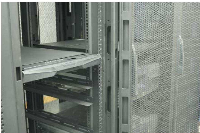
Figure 7. Pushing the LCD drawer until it is located in the rack.
