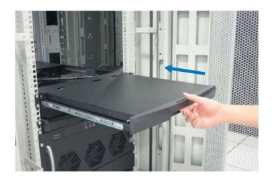
■ Press the handle button and gently push back the drawer into the rack.
