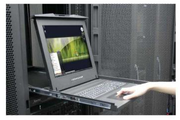
Figure 6. Operating the LCD keyboard drawer.
