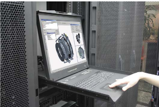
Figure 6. Operating the LCD keyboard drawer
