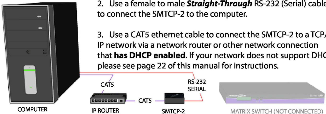
2. Use a female to male ***Straight-Through*** RS-232 (Serial) cable to connect the SMTCP-2 to the computer.
