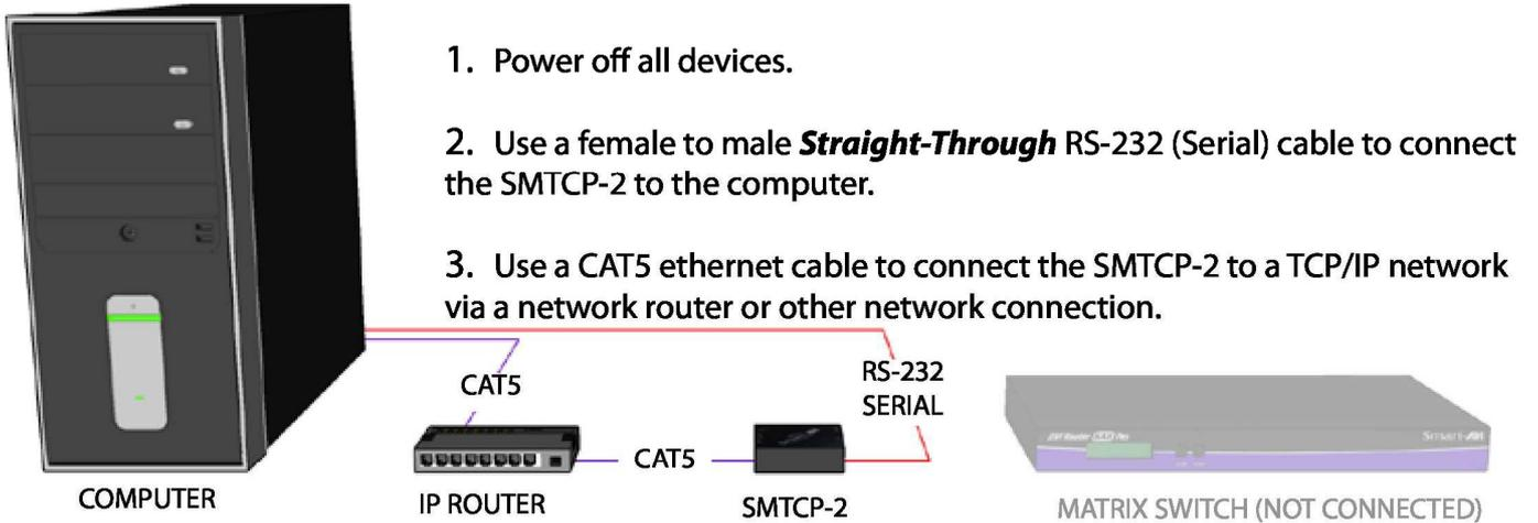
4. Power on the computer and run a terminal program such as Hyperterminal to open a serial connection to the SMTCP-2 using the standard 9600 baud, 8, N, 1, None Flow Control configuration.
