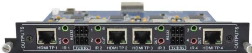
Provision is made within the card for passing RS-232 and IR over the same CAT5 cable. These are specific to the HDBaseT channel. They do not have to be used for the HDBaseT channel to function, but are provided for those situations where they are needed. Please note that this is separate of the RS-232 and IR channels that are provided for the MVID-MTX Matrix unit's controls.
