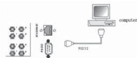
Users can control the MVID-MTX matrix via control software installed in a computer. This requires connecting the RS-232 port on the back of the matrix chassis to a serial RS-232 port on the computer. To control the switcher, users need a Terminal Emulator such as Hyper Terminal installed on the computer.
