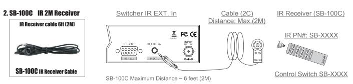
The SB-100C IR Receiver will not function on the port "ALL in" Jack.
