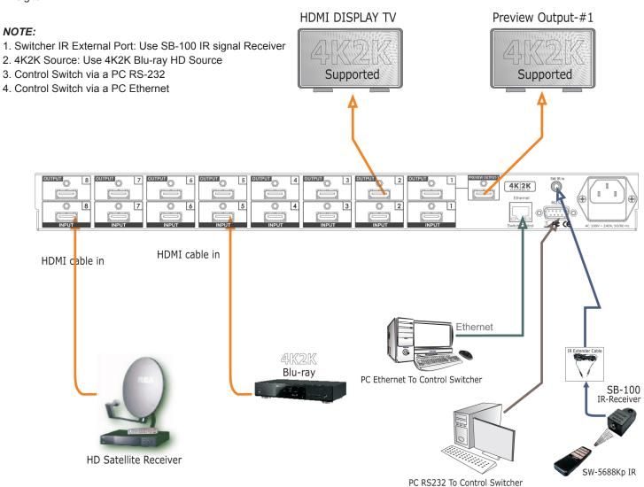
Application RS-232, IR and Ethernet to control the switcher.
