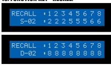
The system will show previously stored presets, up to a total of (16). Presets are stored in local memory using Source keys 1 thru 8 or Destination keys 1 thru 8 as the memory preset location.
