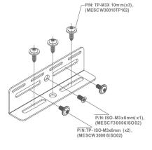
Model No.: #4U-10p-M130MM-EAR SB-6335T/R 4U Ear mount pairs Parts No.: MEER6335ER11001
