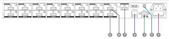
1. DC POWER INLET: The Switcher is fitted with an AC power plug input connector. Ensure that the used is of an approved type and is of sufficient current carrying connector capacity with the correct voltage and connector polarity. 100~240Volt AC, 50/60Hz power supply.
