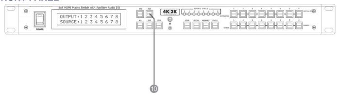
10. FUNCTION KEY - AUX (The audio additional on the "Audio / ARC" port )
