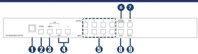
IR Window: IR receiver for signal from the device's remote control or external IR controller
