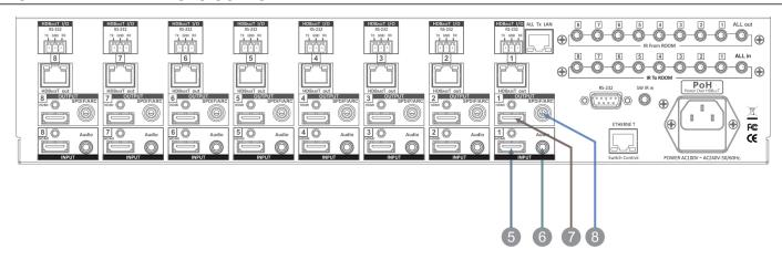
**5. INPUTS-1,2,3,4,5,6,7, & 8 HDMI:** Connects a HDMI signal source direct to the HDMI digital video/audio female HDMI connector. This HDMI port supports HDMI and DVI digital video sources. If you remove the HDMI screw posts, you must use the provided HDMI Locking Post replacement screws to keep the internal HDMI jack secure. Removing the HDMI screws without installing the HDMI Locking Post replacement screws will void your warranty.
