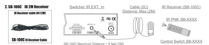
The SB-100C IR Receiver will not function on the port "ALL in" Jack.
