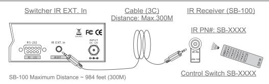
The SB-100 IR Receiver is required when using the port "ALL in" Jack.
