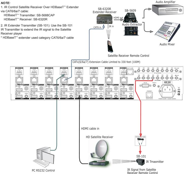
Supports HDBaseT™ Extender by Switcher Transmitter and SB-6320R Receiver via CAT6/6a/7 cable.
