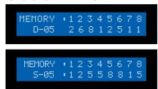
The system will show stored presets, up to a total of (16). Presets are stored in local memory using Source keys 1 thru 8 or Destination keys 1 thru 8 at the memory preset location.
