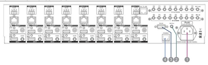
**1. DC POWER INLET:** The switcher is fitted with a AC power plug input connector. Be sure it is an approved type and is of sufficient current carrying connector capacity with the correct voltage and connector polarity. 100~240Volt AC, 50/60Hz power supply.
