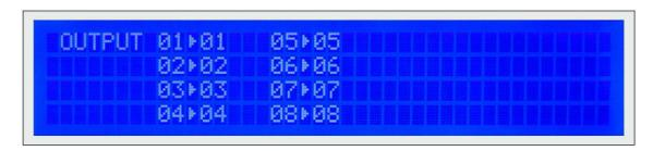
To assign an output to an input, press SWITCH. A blinking block cursor will appear. Use UP and DOWN to select the input that you would like to assign. Once the cursor is over the desired input port, press ENTER to enter editing mode. Press UP and DOWN to select the output port. Once you have selected an output, press ENTER to save the configuration. To escape from editing mode, press ESC.
