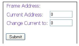
The frame address menu allows you to set the frame address of the current matrix switch. Frame addresses allow commands to be sent to different matrixes in series. For more information on the specific commands available, please see the instructions for your matrix switch.
