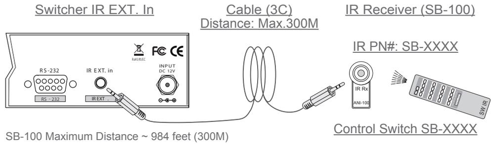
The SB-100 IR Receiver is required when using the port "ALL in" Jack.
