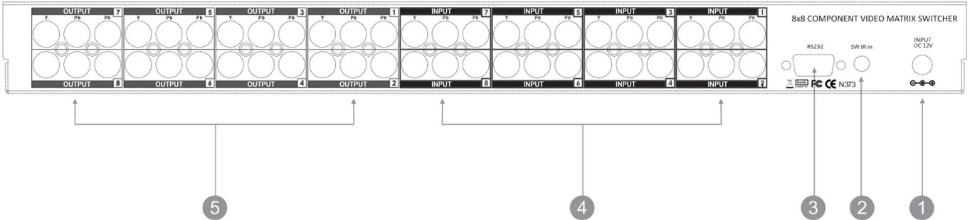
**1. DC POWER INLET:** The switcher is fitted with a DC power plug input connector. Please ensure that the plug used is of an approved type and is of sufficient current carrying capacity with the correct voltage and connector polarity. 12Volt DC power supply 2A Max.
