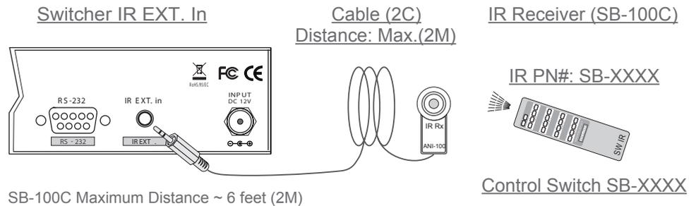
The SB-100C IR Receiver will not function on the port "ALL in" Jack.
