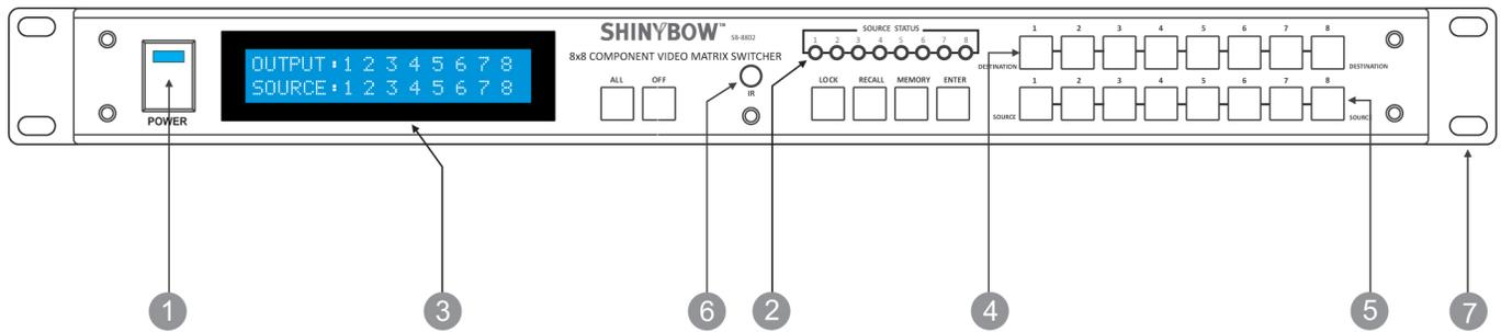
**1. POWER ON SWITCH:** The power switch turns the unit on and off. The LED will illuminate red to indicate that the switcher is ON and is receiving power. The switcher will remember that last state during a power cycle. When power is removed and resorted, the last configuration will be evoked.
