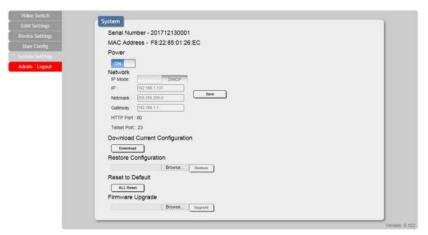
• This page provides system configuration options including turning the unit's power ON/OFF, changing the network settings, downloading/restoring saved system configurations and updating the firmware.
