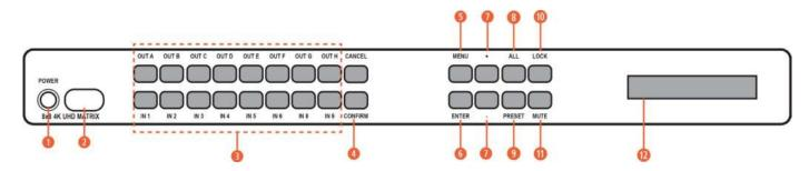
**OPOWER:** Press this button to power the unit on (Green LED) or place it into stand-by mode (Red LED).
